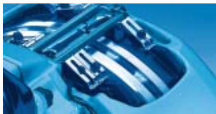
Lining wear indicators (BVA)
