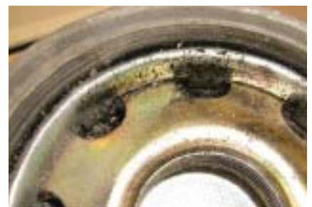
Fig. 2 : Desiccant cartridge with coalescence filter after 60,000 km
